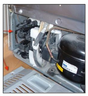
This is the compressor of a kitchen refrigeration unit. It is in the back of the refrigerator.
